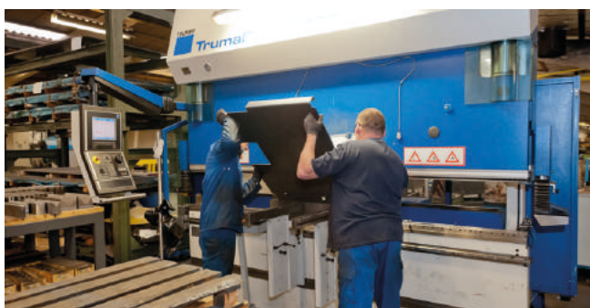
Computer assisted steel plate bending
